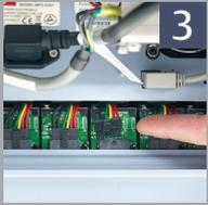
**3** At each connector, firmly grip the cable plug and line the plug up with the socket below it. Insert it until the latch locks completely (the latch should click into place).
