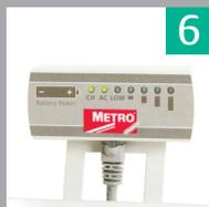
6 During charging, green CH and AC LEDs are on and amber LEDs display charge progress. The AC LED stays on until the cart is unplugged for mobile use. Once charged, the CH LED goes off.
