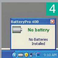
4 Install the Metro BatteryPro software on the computer to view the battery's status, charge level, charge time, remaining runtime and health.
