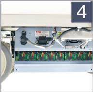
**4** Check that all connections have been made properly. There are 8 battery pack connectors in the Lithium Nano power supply.
