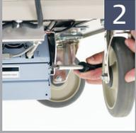
**2** Remove the screw on the sides of the power supply that hold on the battery connector access panel in place and rotate the access panel down.
