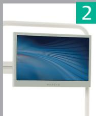
2 Gently push or pull the top of the monitor frame to tilt, swivel or rotate the monitor. If equipped with the articulating arm, you can also raise and lower the monitor height. With the overbridge mount, monitor height can be adjusted by raising or lowering the monitor mounting bar.
