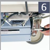
**6** Re-Install the screw on both sides of the power supply that hold the battery connector access panel.
