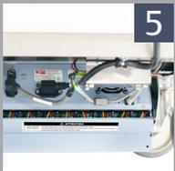
**5** Rotate the battery connector access panel back up, pushing until the top is seated against the case.
