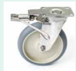
All stainless steel construction. Grease sealed stainless steel ball-bearings with zerk fittings. Available in 6" (152 mm) diameter, swivel, brake-lock and swivel-lock tracking options.
